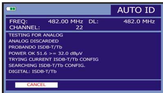
Figure 53.- Automatic identification of the signal.
