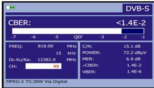
Figure 38.- DVB-S (QPSK) signals CBER measurement screen.
