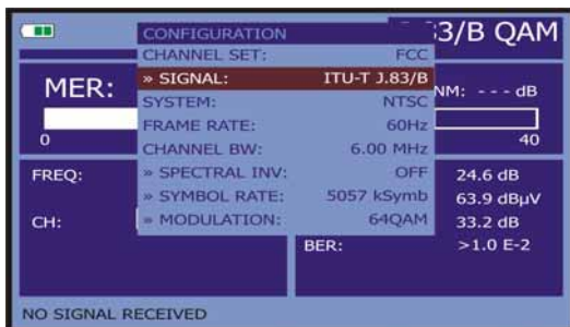
Figure 20.- Screen of measurement configuration (QAM Annex-B signals).
