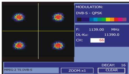
Figure 48.- Constellation Diagram. DVB-S (QPSK) signal.
