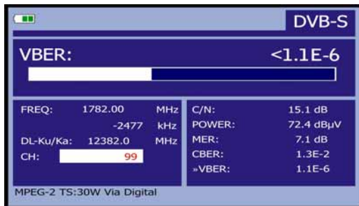
Figure 40.- DVB-S (QPSK) signals VBER measurement screen.
