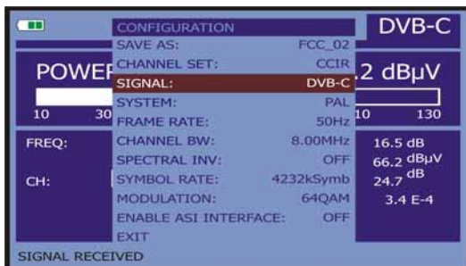
Figure 19.- Screen of measurement configuration (QAM signals).
